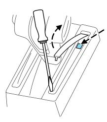
If it is necessary to use the above procedure to move the gearshift lever, it is possible that a fuse has blown or the vehicle's brake lamps are not operating properly. Refer to *Fuses and relays* in the *Roadside Emergencies* chapter.
